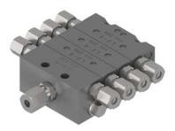
The LX-4 distributor is a modular type progressive metering device and is suitable to be used as a main or secondary distributor. The number and feed rate or the lubrication points can easily be changed as required at any time. The combination of up to 4 outlets is possible. The LX-4 distributors are the alternative for the MX-F with a high metering flexibility.
