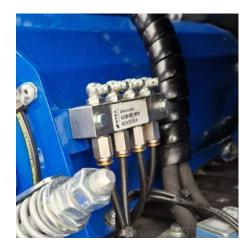
A centralized lubrication system is like having a multi-outlet grease gun. It lets you pump grease from a central reservoir or distribution block to multiple lubrication points on your machine with a single action.
