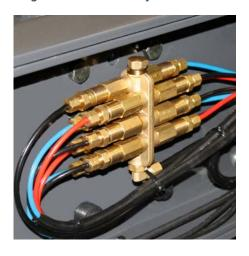
A single-line system consists of a central pump and delivers lubricant through a single line to the metering devices. Each metering device serves a single lubrication point, operates independently and can be individually adjusted to deliver the desired amount of lubricant.
