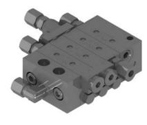
The MX-F distributor is a modular type progressive metering device and is suitable to be used as a main or secondary distributor. The number and feed rate or the lubrication points can easily be changed as required at any time. The combination of up to 4 outlets is possible.
