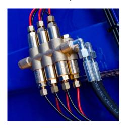
A dual-line system consists of a central pump and delivers lubricant through two main lines to the metering devices. Each metering device serves a single lubrication point, operates independently and can be individually adjusted to deliver the desired amount of lubricant.
