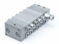
The Groeneveld progressive distributors are a modular type progressive metering device and suitable to be used as a main or secondary distributor. The metering outlets cover a metering volume of 0.025 up to 0.105 cm3 per outlet. The combination of up to 4 outlets is possible.
