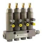
The BEKA BL-1 metering units for single line systems can be combined with up to 6 metering valves per manifold. Metering can be adjusted for each lubrication point at each distributor. The BL-1 has an adjustable metering volume of 0.2 up to 1.2 cm3 per stroke and outlet. Up to 3 valves of the BL-1 can be bridges to get a higher output.
