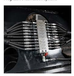
A progressive system consists of a pump and delivers lubricant via a main line to a progressive metering devices. The progressive metering device supplies the lubricant to the lubrication points in inevitable order.
