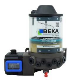
The BEKA PICO combines power and flexibility with a compact design. The PICO system offers the unique combination of progressive- and multi-line technology in one system, with 2 progressive outlets and up to 8 outlets for point to point lubrication. The PICO is ideal for small machines with approximately 20 lubrication points.
