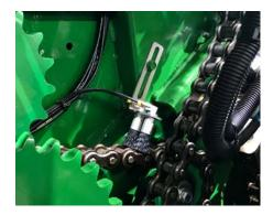
Different types of brushes are available to meet the different requirements of applications as lubrication systems for chains or surface wetting. Brushes do not only lubricate the contact points of the links, but rather the entire chain. Brushes are available in different sizes to suit different chain dimensions.
