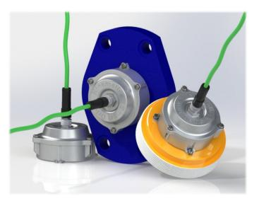
The Smart Drive / WG encoder (Worm and Gear Encoder) is available as absolute, multiturn and single-turn encoders installed to the Kinematics slew drive as the newest addition to the Kinematics Smart Drive ecosystem. These encoders are capable of absolute accuracy of greater than 0.1° per turn and output unique positional data for up to 20,000 turns. Being an absolute encoder, the WG series encoder is able to provide accurate and reliable positional data of your drive even if power is lost.
